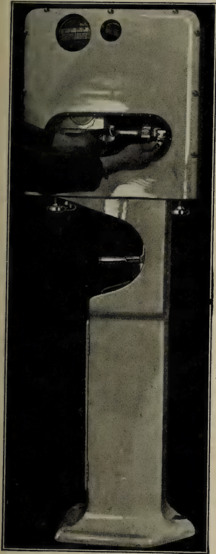
Fig. 101. Removing Wire and Rod from Scale Beam. This allows the scale beam to move freely.
